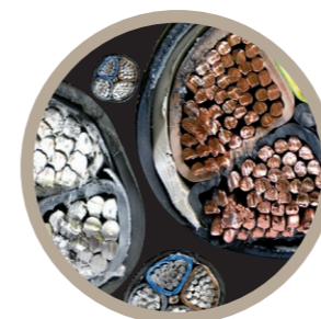
5 Energetski kabeli 1-30 kV
